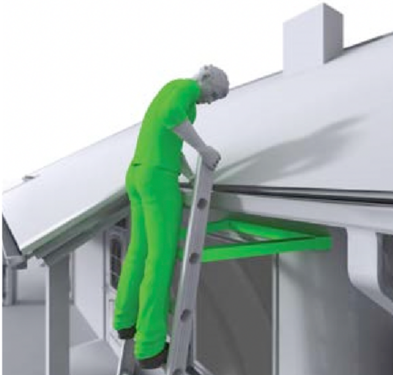
Figure 4 Correct – use of a stand-off device to ensure a strong resting point. Do not rest a ladder against weak upper surfaces such as glazing or plastic gutters. Follow the manufacturer’s instructions
